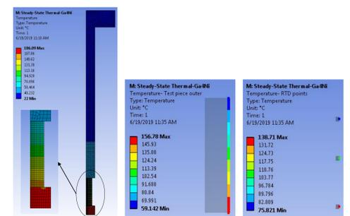
Steady State Temperature Results from FEA for *Ga<sub>4</sub>Ni*: (a) Full Model, (b) Outer Surface, and (c) at RTD Points
