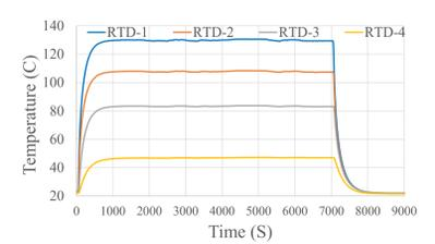
Temperature Plots from Low Carbon Steel Test
