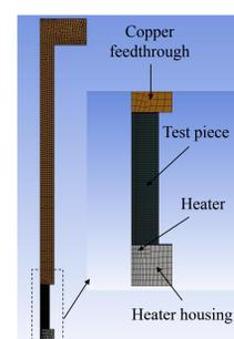
Axisymmetric Finite Element Model of the Test.
