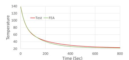
Comparison of Cool Down Temperature Results Obtained from Test and FEA for RTD-1
