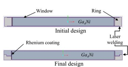
Capsule diameter and thickness = 2.750" and 0.220", window thickness = 0.012"
