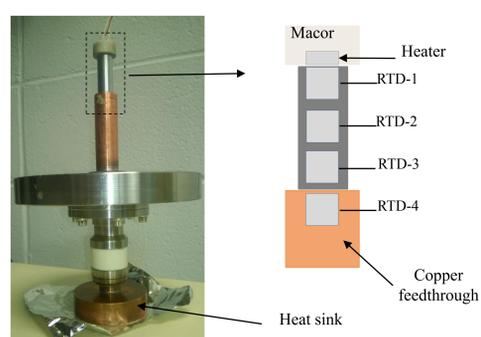
*Ga<sub>4</sub>Ni* Test Piece Preparation for the Test
