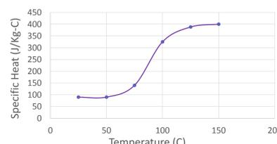
Specific Heat, *C* of *Ga<sub>4</sub>Ni* Obtained from the Test and FEA
