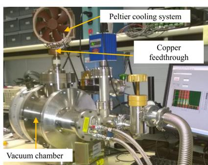
Experimental Test Setup
