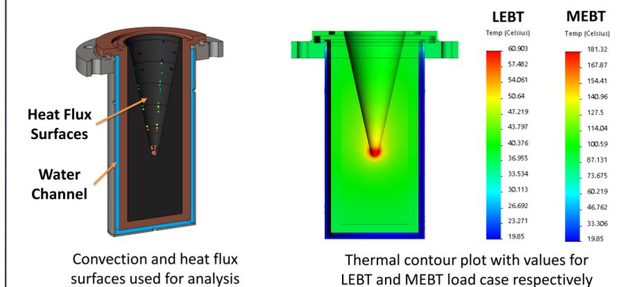
Convection and heat flux surfaces used for analysis Thermal contour plot with values for LEBT and MEBT load case respectively
