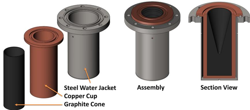
Individual components of the Faraday cup, assembly, and internal section view
