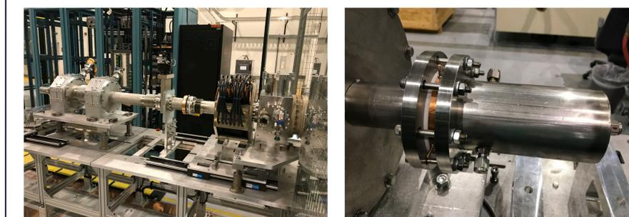
H<sup>+</sup> RFQ Test Stand LEBT assembly Faraday cup located at the beamline end
