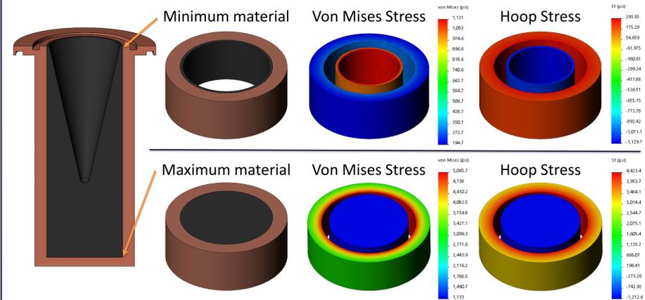
Two conditions for interference fit Deformed stress contour plots for each case
