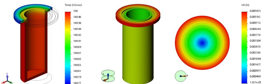
Thermal contour plot from heating Radial displacement contour plots about center axis
