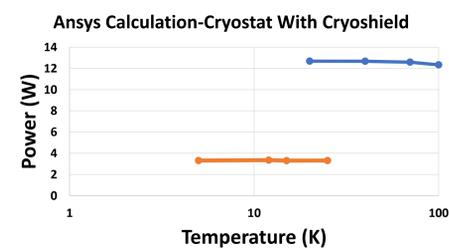
Shield added, Ansys calculation of cryostat cooling required. Cathode temperature reaches 15 K.
