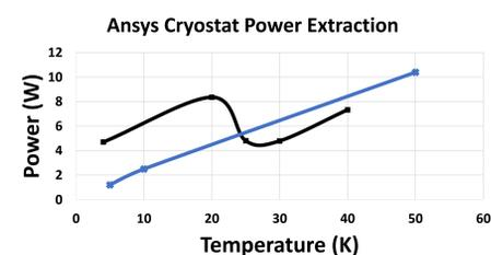
No shield, cryostat power extraction comparison. Cathode temperature reaches 40 K.
