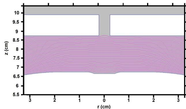
With  $V = -200$  kV applied to the electrode, we find that  $E_{max} = 11.05$  MV/m on the shell.
