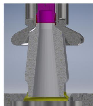
Stainless Steel collar shielding the thin ceramic.
