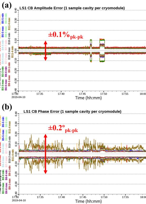
Figure 4: Measured amplitude and phase errors with beam: (a) fractional amplitude, (b) phase. The measurements are the same as shown in Fig. 3, but with a time span of 30 minutes and two intervals with the high-peak-current pulsed beam on. The beam was accelerated at 17:47 (for  $\sim 20$  seconds) and 17:49 (for  $\sim 90$  seconds).
