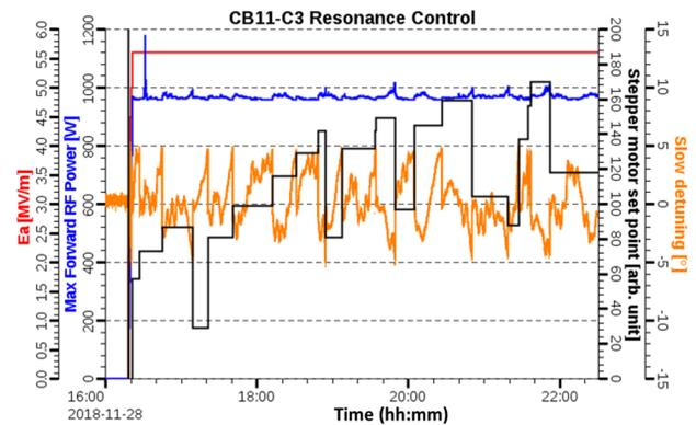
Figure 5: Resonance control of a  $\beta = 0.085$  QWR at 4.5 K. The slow detuning (orange) is the phase difference between the input and pickup RF signals, filtered by a 3 Hz low-pass filter. The peak forward RF power (blue) is measured every second with a 100 kHz bandwidth. Red: accelerating gradient. Black: stepping motor position set point.
