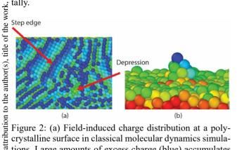
Figure 2: (a) Field-induced charge distribution at a polycrystalline surface in classical molecular dynamics simulations. Large amounts of excess charge (blue) accumulates at protruding features, such as step edges. Very little charge (green) accumulates in depressions or down from protrusions. (b) Spontaneous formation of a surface nano-tip under a very high electric field (10 GV/m). Ions are emitted from the tip soon after.
