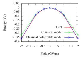
Figure 1: Comparison of the energy of a (100)-oriented copper slab, obtained by density functional theory and by two classical models. Other surfaces show similar agreement with the same set of parameters.
