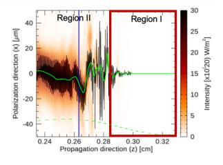
Figure 1: Laser intensity plot at propagation distance  $z=0.229~\rm cm$ . The laser propagates to the right. The averaged centroid (green curve) and non-averaged centroid (black curve) are shown. The green dash line at the bottom shows the laser's initial intensity profile. The laser is self-modulated in Region I (the red box) and it becomes unstable in Region II. The blue vertical line in Region II represents the onset of hosing-like motion at this time.
