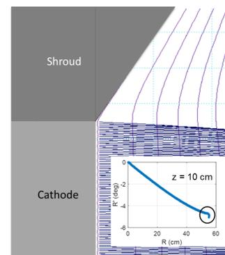
Figure 1: The phase space nonlinearity at the beam edge exists in the absence of an anode hole or magnetic fields, indicating that the cathode/shroud interface is a source.
