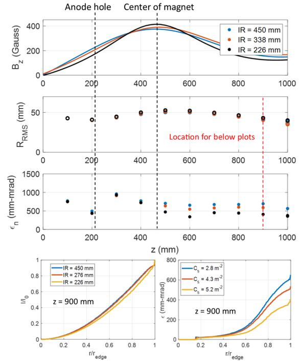
Figure 5: Reducing the magnet radius improves the emittance while maintaining the same beam radius and distribution. This is because the spherical aberration of the magnet fringe fields compensate for the spherical aberration of the anode hole. A magnet with a smaller radius has a larger spherical aberration. The dashed lines indicate where the anode hole and magnet center are located.
