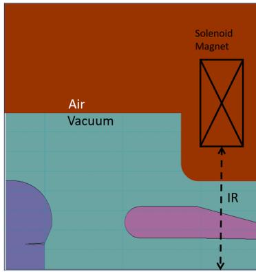
Figure 4: Scale drawing of the injector diode region showing how the radius of the solenoid focusing magnet can be adjusted.
