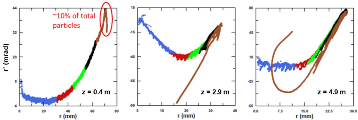
Figure 2: The nonlinearity, representing 10% of the beam, greatly degrades the beam quality as the beam propagates through the injector. Simulation was performed in Amber. Cathode surface is at  $z = 0$ .
