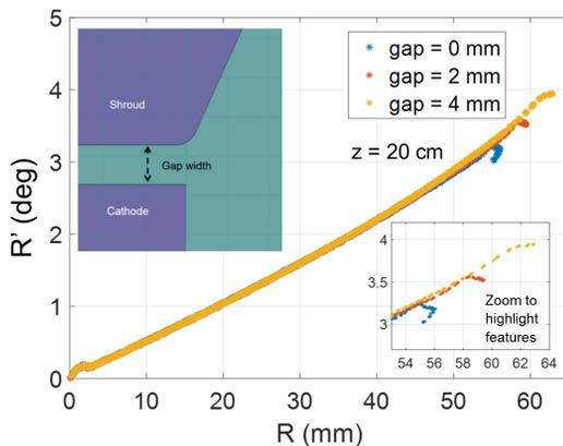
Figure 3: As the gap between the cathode and shroud is opened up, the phase space straightens up at the beam edge. The simulation was performed in Trak with edge emission neglected.
