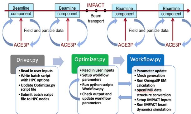
Figure 1: A schematic flow diagram of integrated ACE3P-IMPACT simulation workflow.
