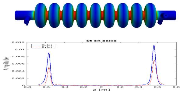
Figure 3: 3D electric field distribution (top) and transverse electric along the axis (bottom) in the boosting cavity.
