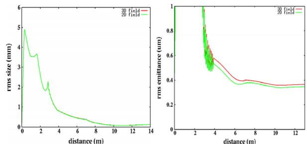
Figure 4: Transverse rms size (left) and emittance evolution (right) through the boosting cavities using the 3D field and the on-axis 2D field.
