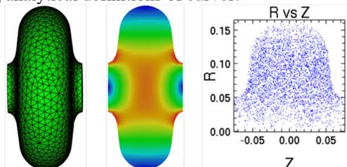
Figure 6: Integrated ACE3P-IMPACT simulation of cavity: (Left) Surface mesh; (Middle) Electric field of operating mode; (Right) Ionized electrons from neon gas.
