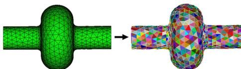
Figure 5: Conversion of surface grid used in ACE3P to individual surface triangles inputted into Warp.
