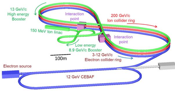
Figure 1: Schematic of current JLEIC baseline design.
