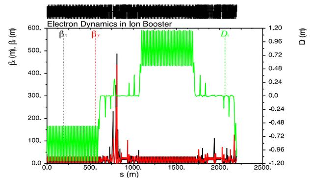
Figure 6: 12 GeV electron beam optics in the new large ion booster, also used as electron ring.
