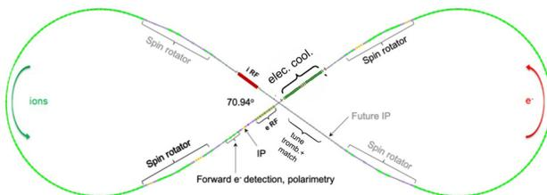
Figure 4: Layout of the new large booster / e-ring with insertions for electrons and ions.
