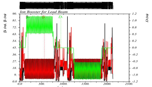
Figure 5: 16 GeV/u lead ion beam optics in the new large booster design with long quads.
