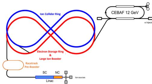
Figure 2: Schematic of the alternative high-energy JLEIC.
