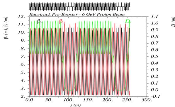
Figure 3: Proton beam optics in the 6-GeV racetrack pre-booster ring.
