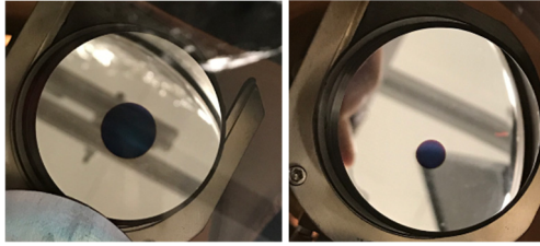
Figure 2: LEReC insertable cathode pucks with deposited cathode material. At the left, cathode of 12 mm diameter on the puck center used during the DC gun commissioning in 2017. At the right, cathode of 6 mm diameter shifted by 4 mm off the puck center is used during LEReC high current operation in 2018 and 2019.
