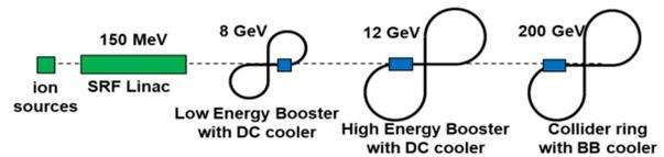
Figure 1: A schematic layout of JLEIC ion complex [3].
