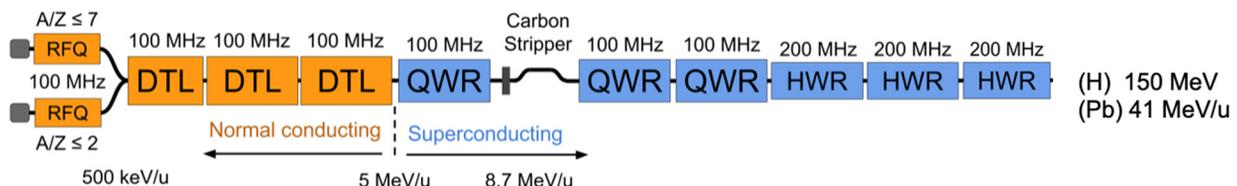
Figure 2: A schematic layout of JLEIC ion injector linac [4].
