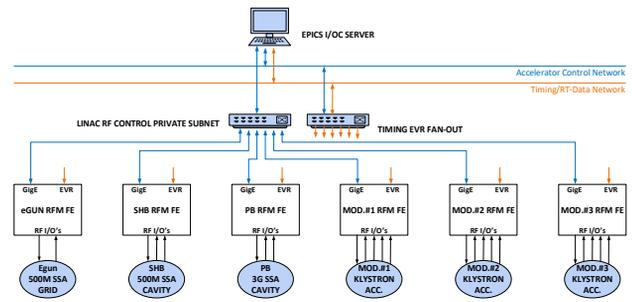
Figure 3: All LINAC RFM nodes are networked in a private subnet within the global control network.
