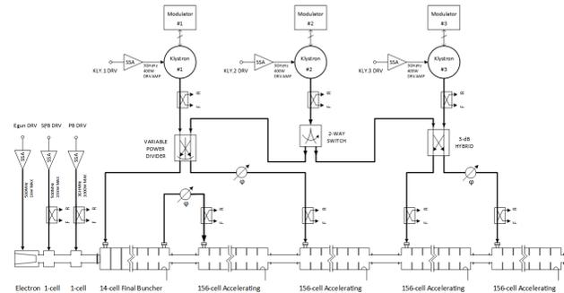
Figure 1: The NSLS-II LINAC rf power plants are comprised of three Solid-State RF PA's for the beam bunchers in the front-end and three 45MW klystrons for the following 4-section 3GHz accelerating structures.
