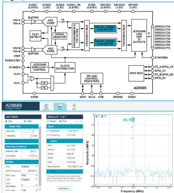
Figure 6: AD9689 Rx\_ADC SNR performance evaluated at 3GHz for the RFM DPD Observation receiver application.
