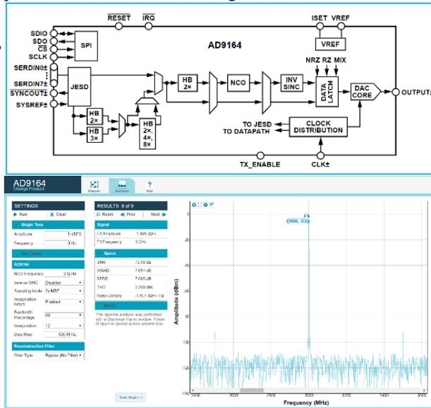
Figure 5: Output spectrum and SNR of AD9164 Tx\_DAC directly synthesizing a 3GHz transmitter carrier frequency with a 6GHz clock and 500MSPS baseband data input.
