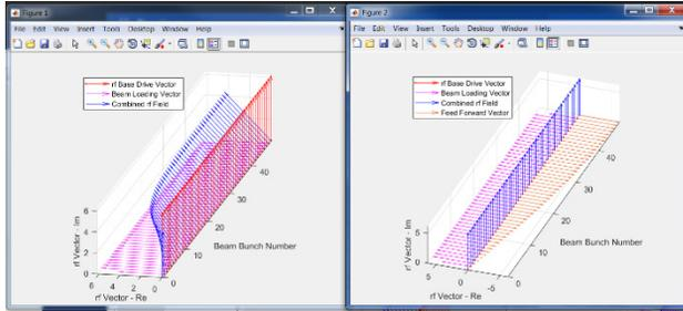
Figure 2: Beam-loading effect of Multi-Bunch beam in the rf field (left) and its compensation with Digital Pre-Distortion (or “feed-forward”) rf modulation (Right).
