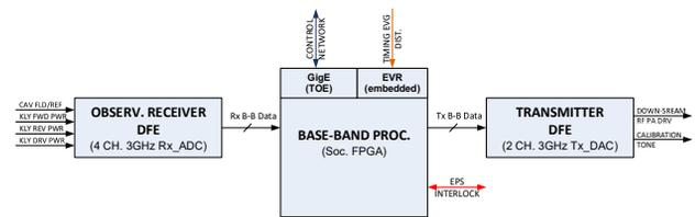
Figure 4: The RFM hardware design is primarily a digital radio (with both Tx and Rx) supported by the interfaces for the control Ethernet and the Timing Event Receiver.
