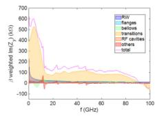
Figure 3: Beta-weighted imaginary part of the vertical impedance, for the individual components and their sum.
