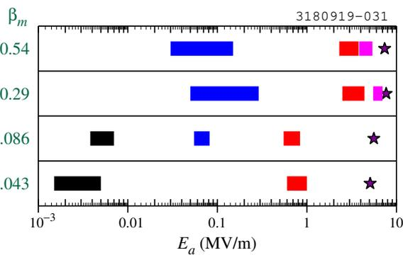
Figure 4: Map of field levels where multipacting barriers are observed in FRIB resonator Dewar tests.
