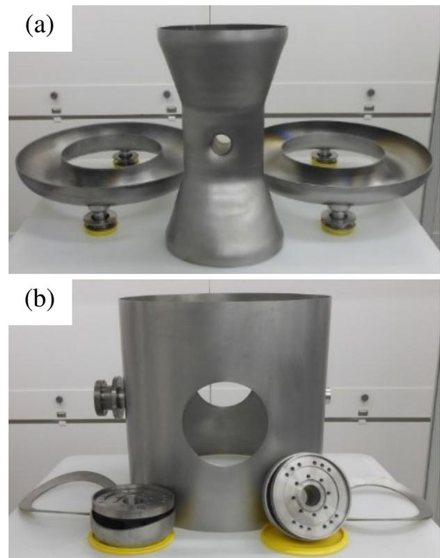
Figure 1: Partially-assembled  $\beta_m = 0.54$  HWR: (a) inner conductor and short plates; (b) outer conductor and beam port cups.
