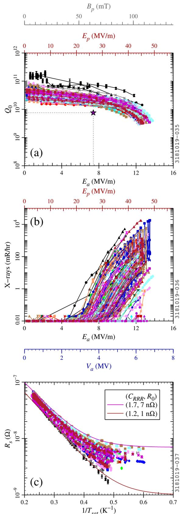
Figure 2: Dewar test results for  $\beta_m = 0.54$  HWRs: (a)  $Q_0$  at 2 K; (b) X-rays at 2 K; (c)  $R_s$  during pump-down. Purple star: FRIB operating goal.
