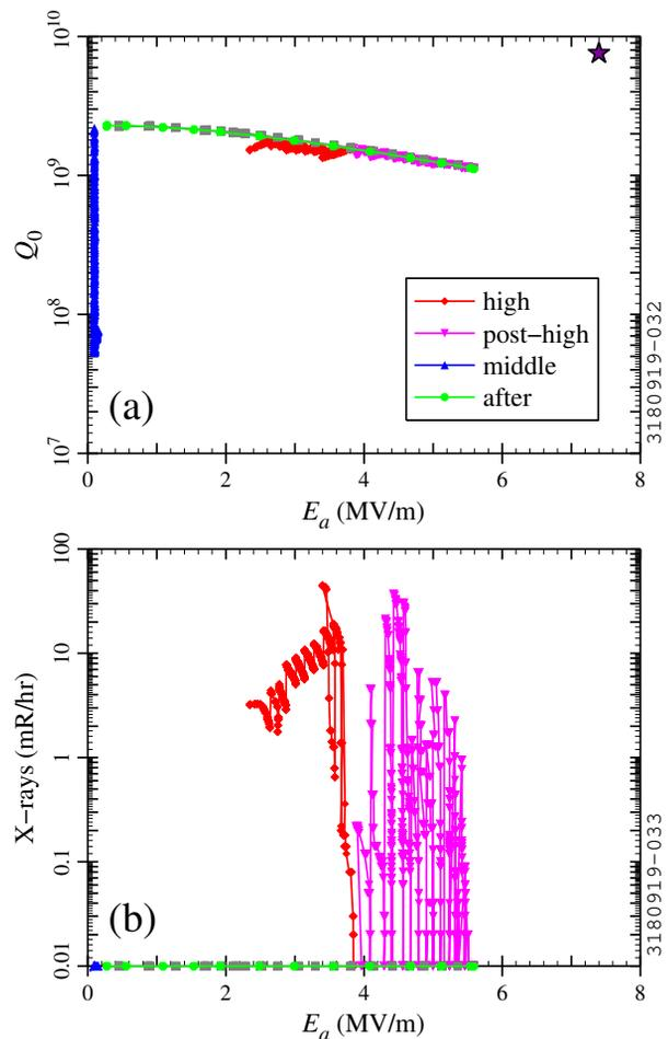
Figure 5: CW measurements at 4.3 K for a  $\beta_m = 0.54$  HWR (S53-091) with MP barriers included: (a)  $Q_0$ ; (b) X-rays.
