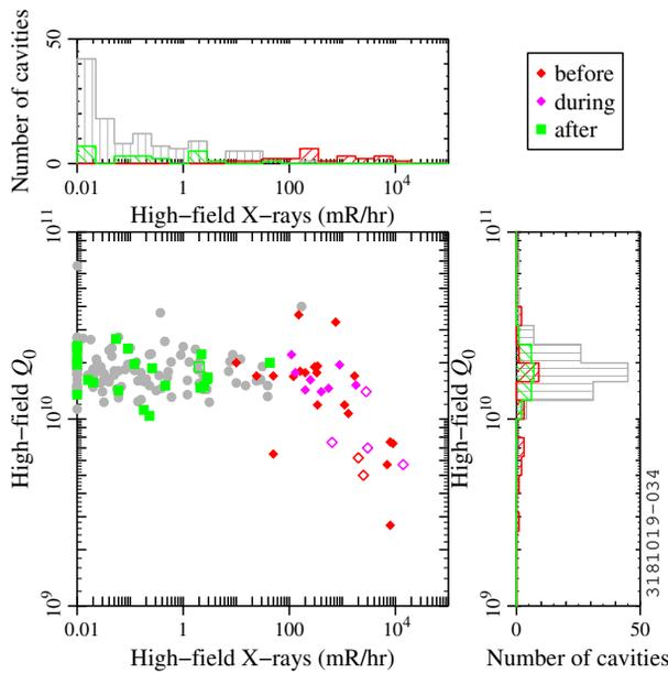
Figure 3: X-ray level and quality factor at high field before and after FE rework for  $\beta_m = 0.54$  HWRs. Histograms of the X-ray level (right) and quality factor (top) are included.
