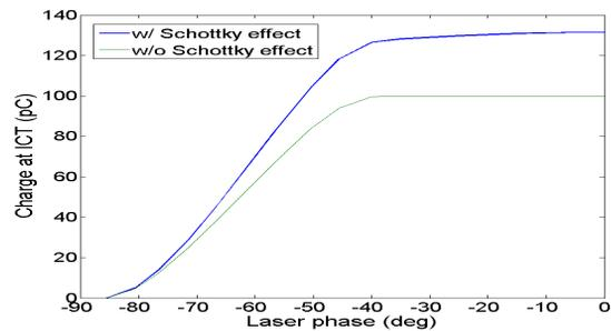
Figure 5: Simulated laser launch phase scan, with and without Schottky effect.
