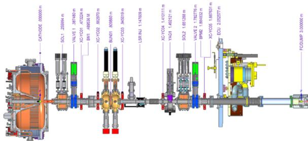
Figure 2: LCLS-II injector layout.
