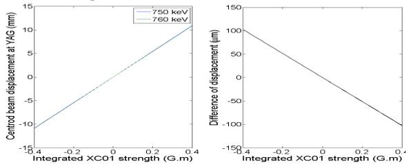
Figure 3: Simulated beam position versus corrector strength for both 750 keV and 760 keV (left), and difference between these positions versus strength (right).
