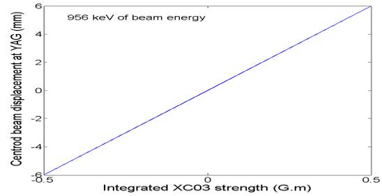
Figure 4: Simulated beam position versus corrector strength for buncher energy measurement.
