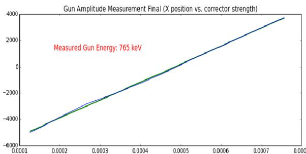
Figure 9: Beam-based measurement of gun energy. Y axis is horizontal beam position on YAG (in microns), X axis is XC03 corrector strength (in kG-m).
