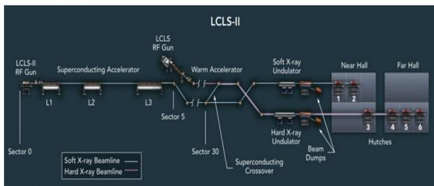
Figure 1: Schematic of LCLS-II upgrade.
