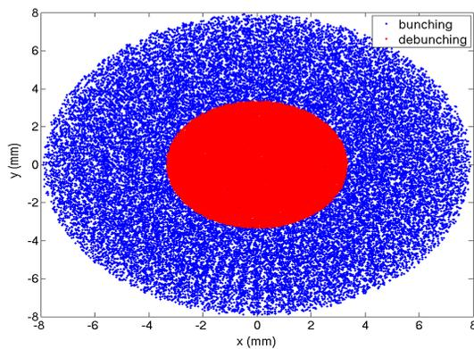
Figure 7: Simulated beam size at YAG screen for bunching and debunching zero crossings.
