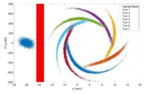
Figure 4: Injected beam position at the injection septum.
