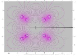
Figure 1: Field Map of the Nonlinear Kicker. The vertical lines show the zero field and maximum field locations on the horizontal axis.
