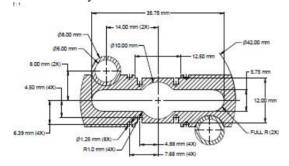
Figure 2: Preliminary design of the vacuum chamber.
