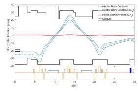
Figure 3: Trajectory of the injected beam from the septum to the nonlinear kicker.
