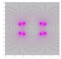
Figure 5: Field Map of the Large Aperture Nonlinear Kicker required for two kicker injection.
