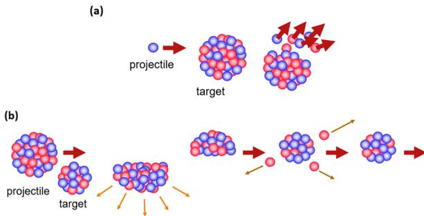
Figure 3: Sketch of (a) ISOL and (b) IF reaction mechanisms.
