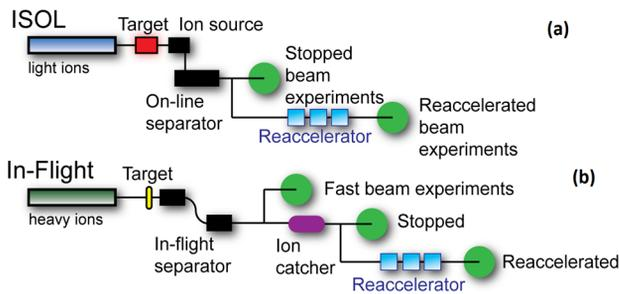
Figure 4: Illustration of (a) ISOL and (b) IF acceleration and separation layout.
