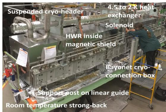
Figure 9: Partially assembled FRIB  $\beta=0.53$  SRF cryomodule.
