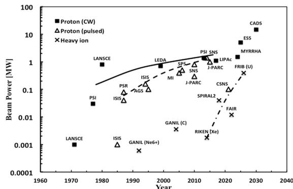
Figure 8: Hadron accelerator beam-power evolution [4].
