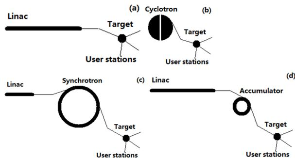
Figure 7: Common high-power accelerator layout of long pulse or CW driven by (a) linac and (b) cyclotron and short pulse driven by (c) synchrotron and (d) accumulator.
