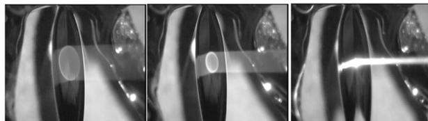
Figure 12: Liquid lithium film intercepting a proton beam of ~60 kV for beam power survival test [46].
