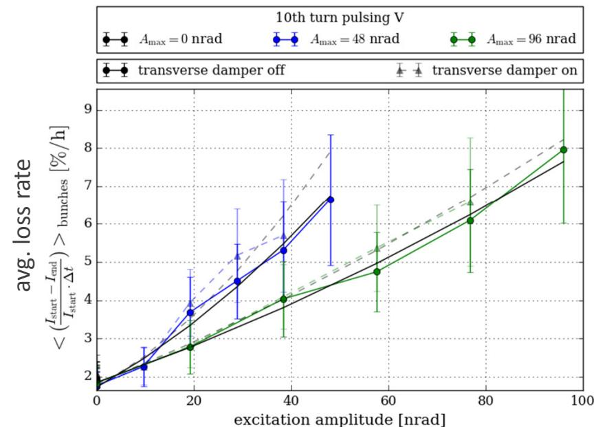
Scaling of losses from fast beam current transformers with excitation amplitude:
