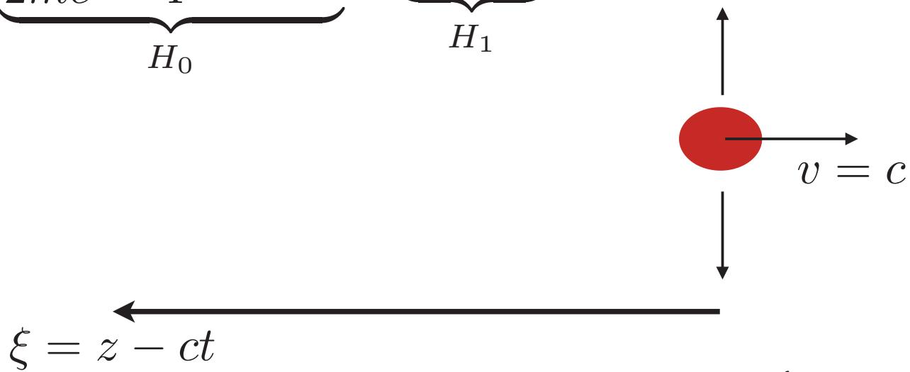
$$E_r(r) = \frac{Ne}{4\pi\sigma_b^2\ell_b} \begin{cases} \frac{r}{\sigma_b} & r < \sigma_b \\ \frac{\sigma_b}{r} & r \geq \sigma_b \end{cases}$$
