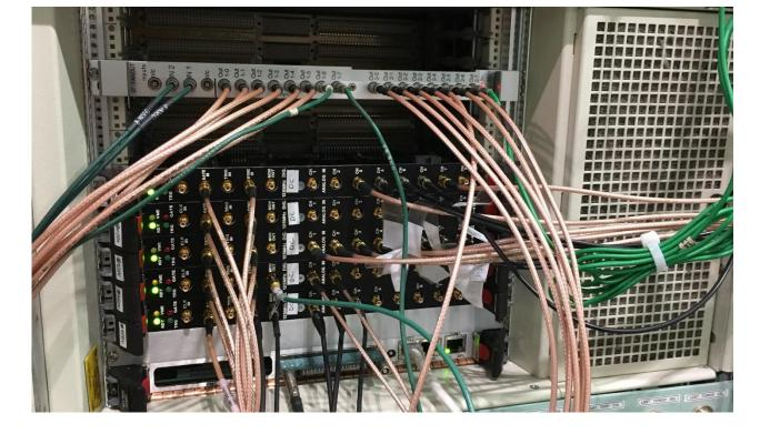
VME based electronics and timing signal fan-out
