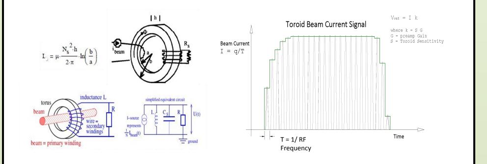
The toroidal pickup follows basic transformer theory. Passing through the center of the toroid, the beam forms a single-turn primary coil of the transformer. The induced voltage is measured across a burden resistor which terminated the secondary coil.
