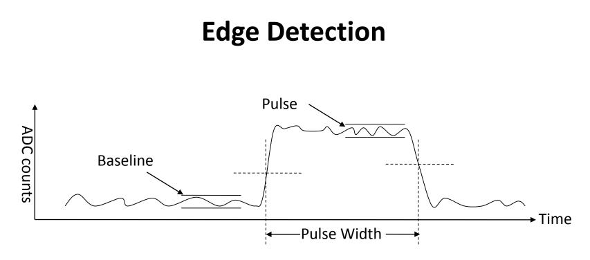
A buffer records the variation of the baseline/pulse. When input samples exceed the recorded range by a predetermined threshold, the edge is detected.
