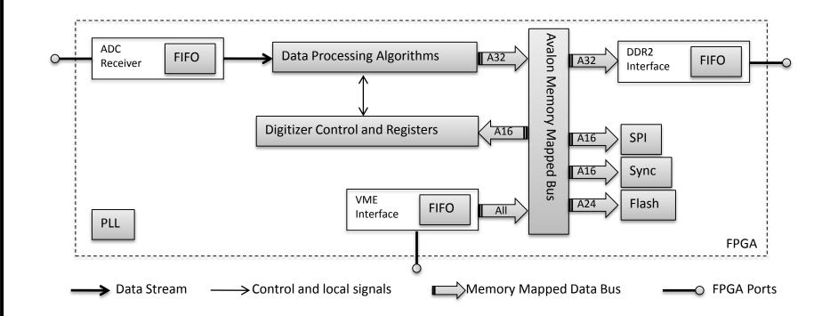
The firmware contains I/O interfaces including the ADC interface, VME bus driver, memory interface, serial interface, etc. as well as application specific algorithms. The connection between the design blocks was developed using the Qsys tool provided by Altera.
