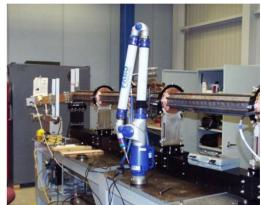
Figure 5: Linac structure on strong-back with supports and portable CMM.
