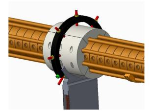
Figure 8: Conceptual model of a wider four-cell saddle.
