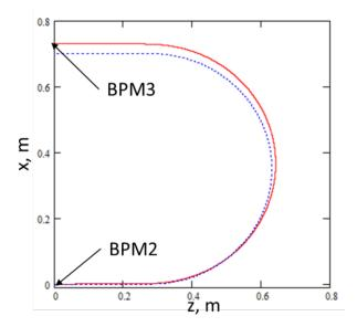
Figure 5: 5% off energy beam trajectory (solid red line) and reference on-energy beam trajectory (dotted blue line) in the realistic soft-edge dipole. The simulations of the off-energy beam trajectory include all the errors listed above.
