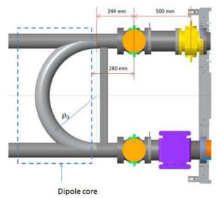
Figure 2: Schematics of 180° bend.
