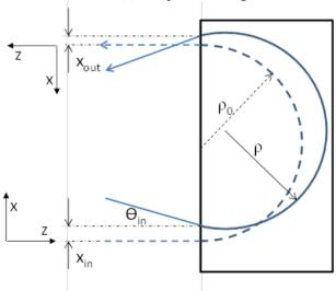
Figure 3: Beam trajectory in 180° bend.
