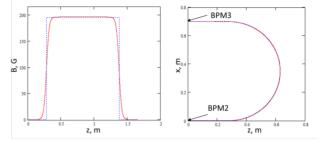
Figure 4: Dipole magnetic field along e-beam trajectory (left) and e-beam trajectory from BPM 2 to BPM 3 (right). The solid red line represents simulation results for the realistic soft-edge dipole. The dotted blue line represents simulation results for equivalent the hard-edge approximation.
