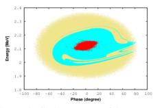
Figure 3: Longitudinal acceptance of the PIP-II SC linac (cyan) with  $6\sigma$  beam at upstream of the linac (red). Initial particle distribution is shown in khakee.
