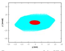
Figure 5: Tranverse acceptance of the PIP-II SC linac (cyan) with  $6\sigma$  beam at upstream of the linac (red).
