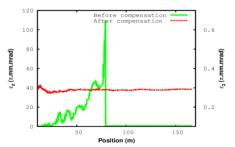
Figure 8: Normalized RMS longitudinal emittance before (green) and after (red on secondary y-axis) applying the local compensation scheme
