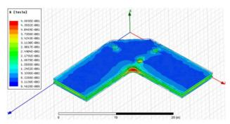
Figure 8: ANSYS Maxwell 3D result for magnetic field map of flag plate of 700-kW design each carrying 50-kA, DC in the opposite direction (+ -).
