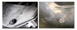
Figure 4: Fatigue failure location of the flag part of the 700-kW high-current stripline [1].
