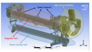
Figure 1: 3D model of the attached magnetic horn 1 (red section), the 700-kW high current stripline (yellow section), water cooling tank (blue section) and spider supports.
