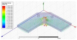
Figure 9: ANSYS Maxwell 3D result for the pressure distribution of flag plate of 700-kW design each carrying 50-kA, DC in the opposite direction (+ -).
