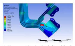
Figure 6: The current density simulation of the flag plate of 400-kW high-current stripline using (half symmetry) using ANSYS Electric.
