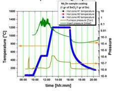
Figure 1: Temperature profile used for coating Nb<sub>3</sub>Sn onto niobium samples. The nucleation process occurs at the first temperature plateau of 500 °C and deposition proceeds at the 1200 °C temperature plateau.
