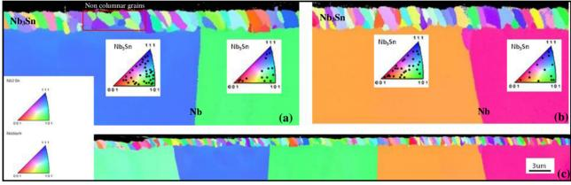
Figure 6: EBSD image of the cross-section from sample U3 is shown in (c). Smaller grains on the top are  $Nb_3Sn$ . Larger grains at the bottom are Nb. Images (a) and (b) are magnified areas from (c). Approximate orientations of  $Nb_3Sn$  grains on each Nb grain are shown with inverse pole figure using assigned color for each grain. Each dot represents an individual  $Nb_3Sn$  grain.
