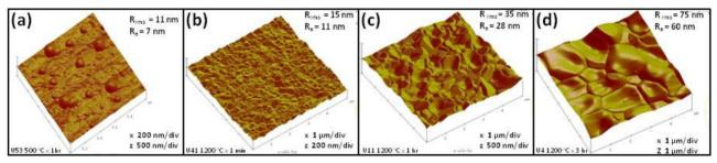
Figure 5: AFM images shows grain growth and topography evolution during the coating process. (a) Sample treated at 500 °C for one hour. The scan size is 1  $\mu$ m x 1  $\mu$ m. (b) Sample treated at 1200 °C for one minute, (c) 1200 °C for one hour and (d) 1200 °C for three hours. The scan size for images (b) – (d) is 5  $\mu$ m x 5  $\mu$ m.
