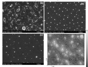
Figure 2: SEM images of samples with a nucleation time of one hour at various nucleation temperatures: (a) 400 °C, (b) 450 °C, (c) 500 °C. EDS was only able to identify tin from bright circular features. SAM elemental mapping of tin coverage from the sample treated at 500 °C for one hour is shown in (d). Note that surface produced after one hour at 400 °C appears very different.
