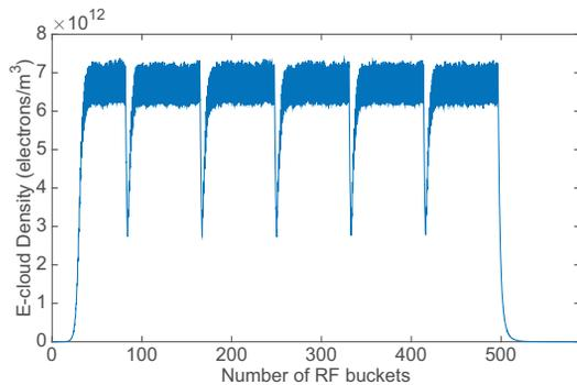
Figure 3: E-cloud density build-up for one turn at 1.9 SEY and  $11 \times 10^{12}$  protons per bunch (field free region).
