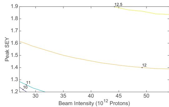
Figure 5: MI dipole region E-cloud density ( $electrons/m^3$ ) contour plot in log scale.
