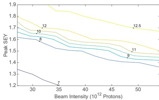
Figure 6: RR field-free region E-cloud density ( $\text{electrons}/\text{m}^3$ ) contour plot in log scale.
