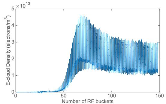
Figure 10: E-cloud density for the Field extraction simulation within a 3mm circle around the vacuum chamber center.
