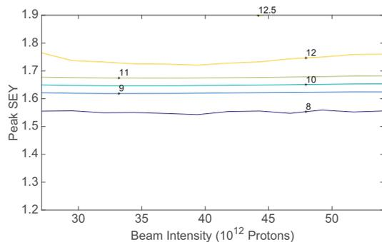
Figure 7: RR dipole region E-cloud density ( $\text{electrons}/\text{m}^3$ ) contour plot in log scale.
