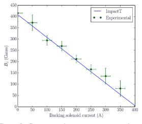
Figure 5: Comparison between IMPACT-T simulations and experimentally recovered values of  $B_{0z}$  from image shown in Fig. 4.
