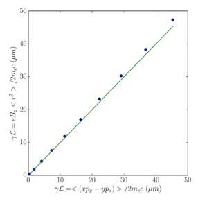
Figure 3: Proof-of-principle via numerical simulations in IMPACT-T of the measurement method. Magnetization  $\mathcal{L}$  is computed from the particle distribution (blue markers) as function of magnetization computed from known  $B_{0z}$  (green solid line).
