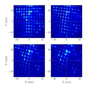
Figure 4: Beamlet formation for (top-right to bottom-left)  $B_{0z}=0$ , 180, 300, 460 Gauss residual field at the cathode observed at YAG2 location. The yellow dashed lines are drawn for reference.
