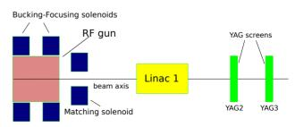
Figure 1: Overview of the AWA witness beamline. The overlap of two solenoid fields produces CAM-dominated beams.
