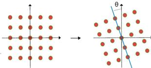
Figure 2: The relative sheering of the beamlet formation due to electron beam magnetization (sketch).
