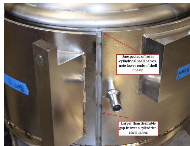
Figure 3: Typical helium jacket fit up to cavity.
