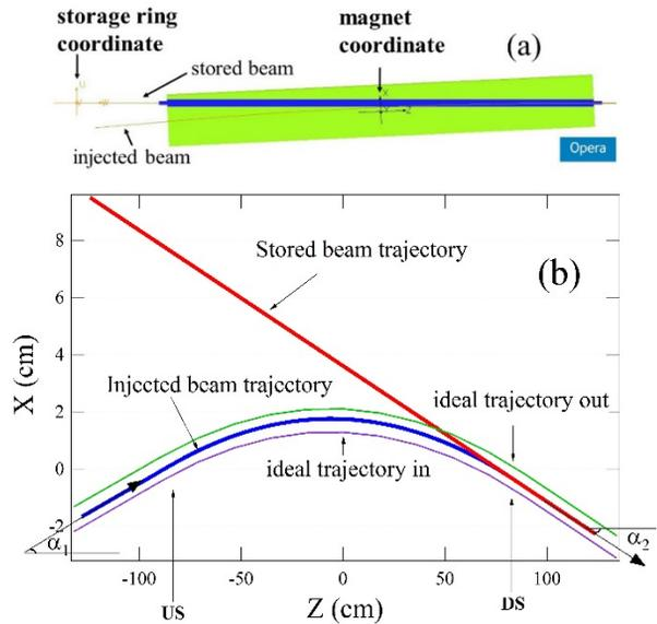
Figure 4: (a) Top views of injected and stored electron beam trajectories of the septum magnet from the storage ring coordinate (all other parts but the bottom pole of the model is hidden); (b) Plots of injected and stored electron beam trajectories from the magnet coordinate. The ideal trajectory in and out show the allowed range of the injected beam in the XZ-plane using an ideal field.
