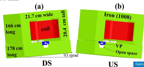
Figure 1: (a) & (b) Views of the septum magnet from the stored beam chamber at the DS and US ends.
