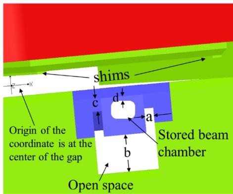
Figure 3: An enlarged view of the stored beam chamber at the DS end. The origin of the coordinate was set at the center of the gap in X, Y, and Z for the modelling.
