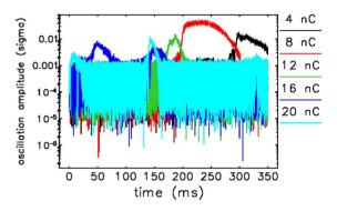
Figure 5: Simulated PAR vertical oscillation at high charge.
