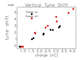
Figure 1: PAR vertical tune shift vs charge. Disabling the pumps increased the pressure by roughly a factor of 2.
