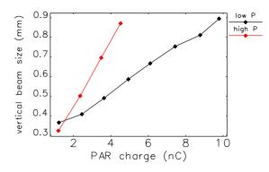
Figure 3: PAR vertical beam size vs charge, with normal and increased vacuum pressure.
