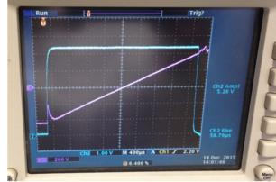
Figure 4: Regulator voltage during a klystron pulse. Ch 2 (blue) shows pulse voltage, 20 kV/div, 400  $\mu$ s/div. Ch 3 (pink) shows regulator voltage, 200V/div, 400  $\mu$ s/div. The pulse settles rapidly and remains extremely flat (< 0.1%) over the long pulse flat top (3.5 ms).
