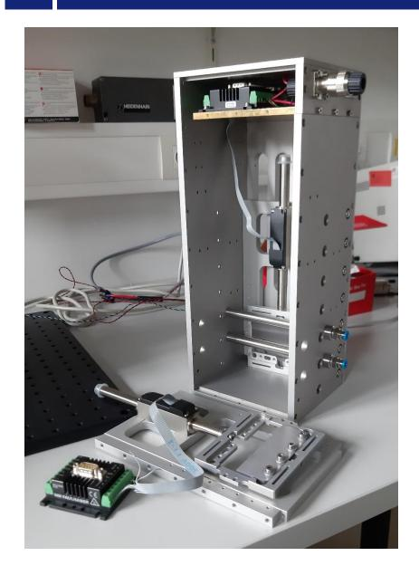
**Modular:** the motors and blades can be assembled in their frames, then onto the cage
