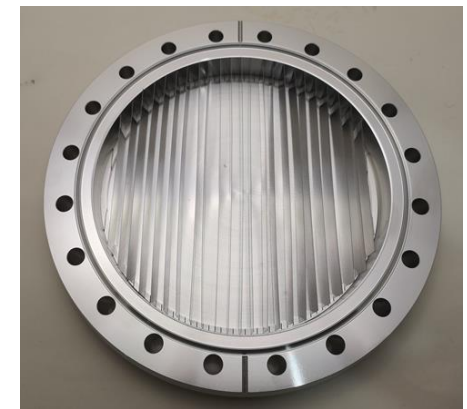
The vacuum vessel for the zero-length CF fin-type NEG pump
