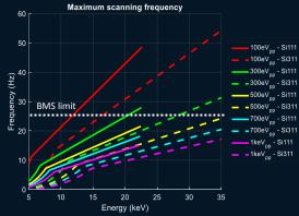
The graphic above shows how rotary stages torque, its encoder and the gap control interferometers limitations impact the system scanning speed, stating boundary curves for each crystal set, central energy and peak-to-peak energy amplitude. For low energies, the interferometer is the main constraint (non-linear in energy), whereas torque (linear in energy) limits the higher frequencies. Scanning frequencies above the curves cannot be performed.
