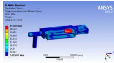
Figure 6: Stress distribution of vacuum chamber
