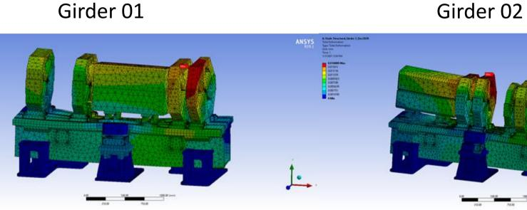
Total Deformation: 0.013mm at magnet top 0.010mm at girder top plate
