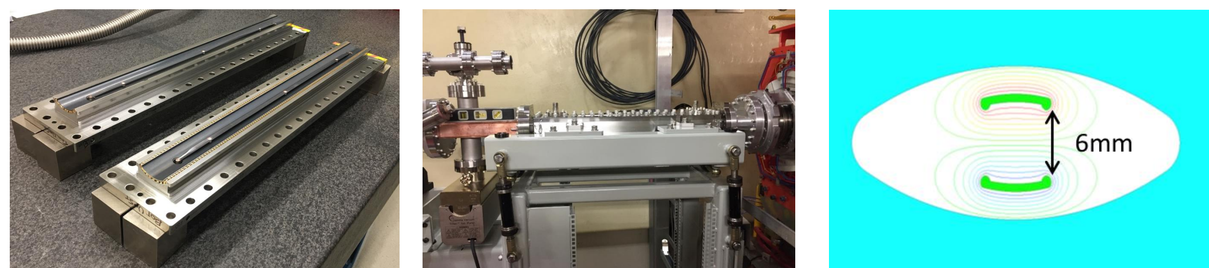
The two side plates of the R&D Kicker with electrodes installed, full assembly in the tunnel and aperture cross section. The R&D Kicker was a vertically kicking beam to avoid wider stored ALS beam size, while the ALS-U will be horizontally kicking with electrodes rotated 90 degrees.
