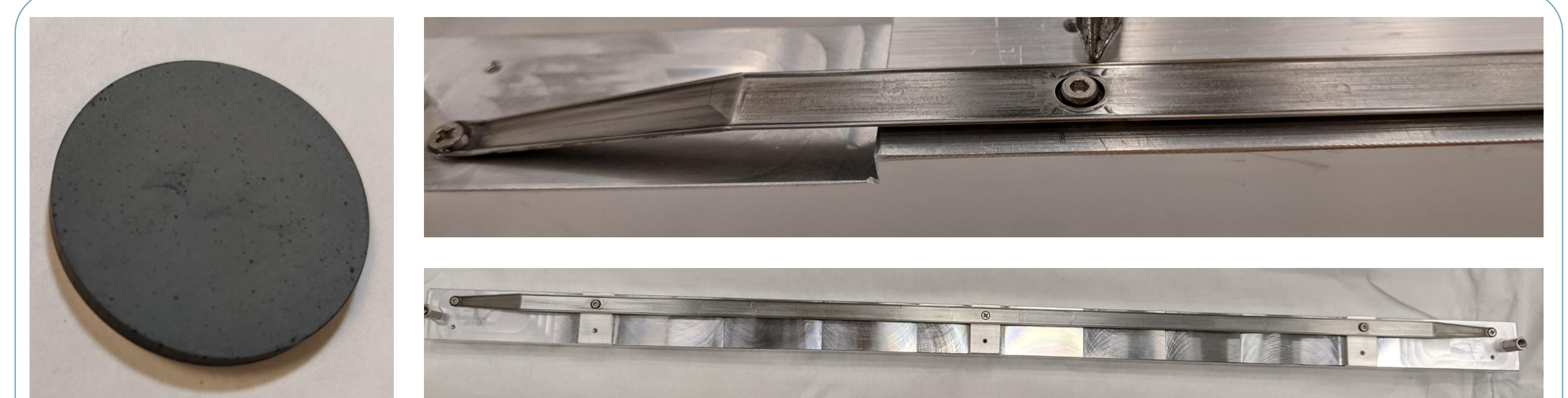
Coated 1" diameter coupon on left and full scale prototype electrode on right. Electrode is cut by wire EDM and then profiled in a CNC. Improvements in CNC programming have reduced tool marks and other witness marks in production of electrodes.
