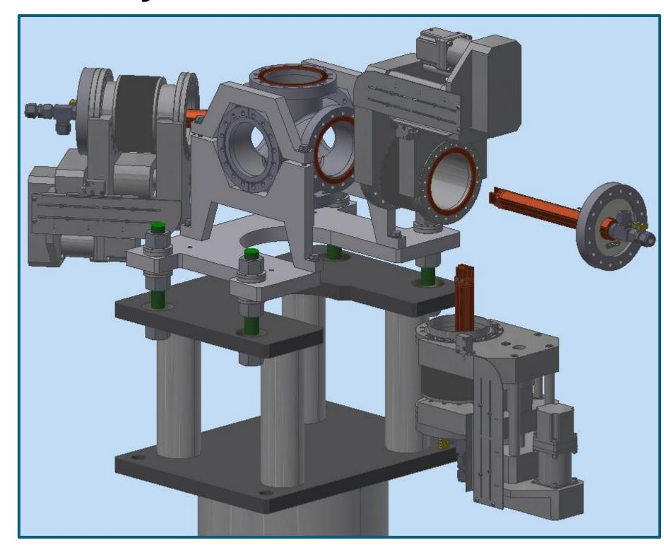
With the SXBPM we aim to achieve micronscale resolution X-ray beam position measurement and accuracy. This requires mechanical stability and detector positioning accuracy on the sub-micron level . The support stand consists of Invar 36 columns capped with steel plates. The BPM is mounted to a leveling plate on top of the stand.
