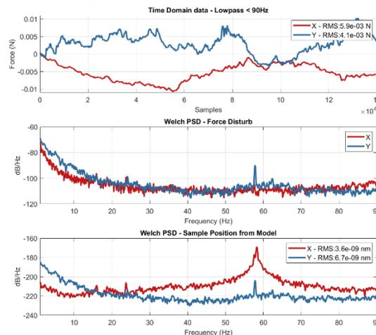
Figure 6: X and Y force time plot and PSD with the referred sample position PSD from the dynamic model.
