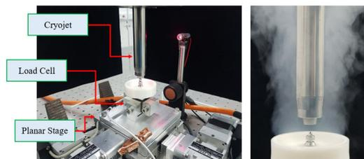
Figure 5: Test setup and mockup shield flow.
