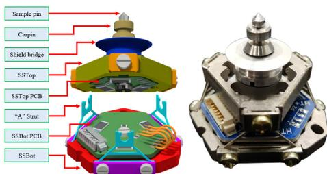
Figure 2: Left: overview of the sample holder with its main subcomponents. Right: picture of the assembly.
