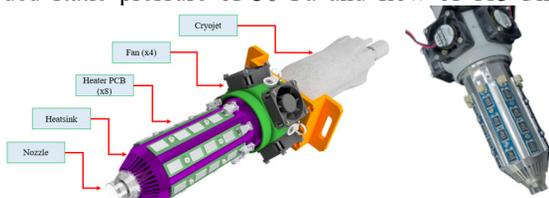
Figure 4: Exhaustion system render and final assembly.
