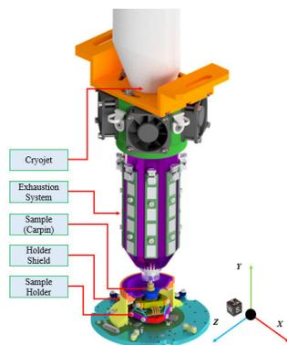
Figure 1: TARUMÃ cryogenic setup main subsystems.
