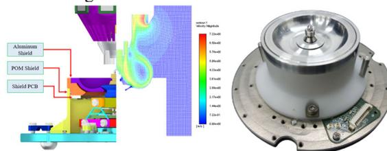
Figure 3: Overview of the Holder Shield including a CFD velocity plot example and the final assembly.
