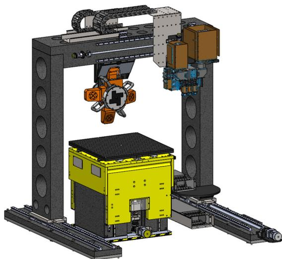
Figure 2: Sample table, detector gantry, tomography microscope and WAXS detector.
