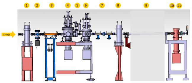
Figure 2: Typical component layout of a hard x-ray front-end at SLS 2.0. Labels: 1. 1<sup>st</sup> XBPM, 2. pump stand, 3 high-power diaphragm, 4. photon shutter, 5. fast- and gate valve, 6. beam stopper, 7. high power slits, 8. 2<sup>nd</sup> XBPM, 9. tunnel wall, 10. pump stand, 11. CVD window, arrow labelled X-Rays: propagation direction of the synchrotron radiation.
