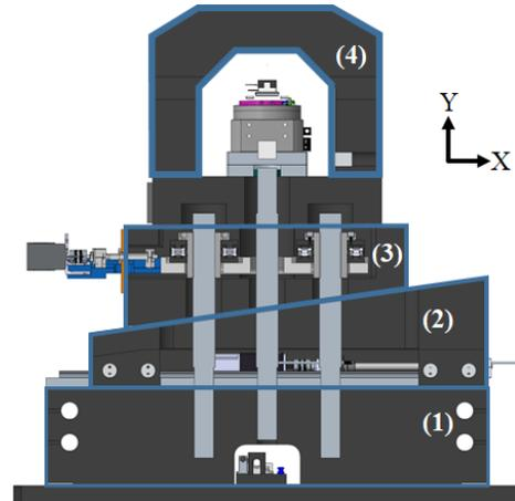
Figure 3: n-CT granite stage stack with motion granite components highlighted. 1- granite Z motion (KZ for sample), 2- X driving wedge that creates Y follower motion, 3- Two degree of freedom Y follower wedge with X motion, 4-Z motion granite gantry for sample environments and detector mounting. Pieces 1, 2 and 3 are nearly identical for supporting the KB system.
