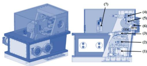
Figure 5: n-CT KB system. VFM – vertically focusing mirror, HFM – horizontally focusing mirror, 1- Vertical stage, 2-Rotation X stage, 3- Translation Z stage, 4- Rotation stage Y, 5-Translation X stage, 6- Rotation Z stage (manual), 7-Clean up slits upstream of the KB mirror.
