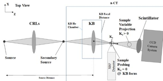
Figure 2: Schematic showing the optical layout and detection of the n-CT instrument. The n-CT works with a secondary source created by a CRL system upstream in the beamline. The new directions KX, KY, and KZ are noted as the “kicked” axes of the beam by the KB mirror pair.
