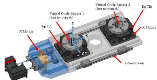
Figure 4: n-CT following wedge guide/drive design. This drive allows the follower wedge to be guided vertically by two posts but be driven transversely.
