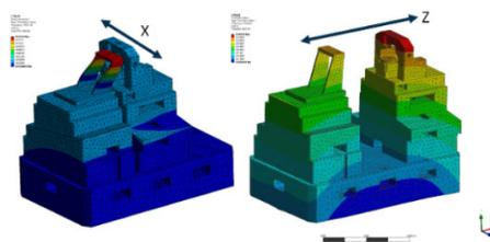
Figure 7: Modal analysis [8] results. The first mode is a KB frame motion (~158 HZ) and is not a rigid body motion of the support structure or granite stages. In the probing (left) and farthest projection position (right), the second natural frequency is ~179 Hz and ~172 Hz respectively for rigid body the rigid body modes. The direction of rigid body motion induced by rocking is shown in the figure.
