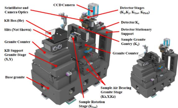
Figure 1: Rendering [6] of the n-CT instrument design, labeling major components. Largest working distance (left) and probing stage (bottom right).
