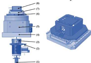
Figure 6: n-CT sample stack. 1-Electrical slip ring, 2- Rotary union separate rotation mechanics, 3- rotary union, 4- base plate, 5-rotation stage, 6- feedthrough manifold, 7- XZ nanopositioner, 8- optional scanning mount or stationary kinematic mount (right picture).
