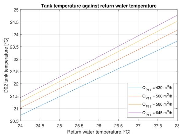
Figure 5: D02 temperature against return water temperature at ST4 nominal conditions.
