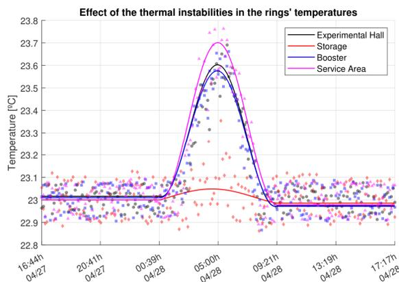
Figure 2: Inlet temperature of the EA, SR, BO and SA rings. Date 28<sup>th</sup> of April of 2021.
