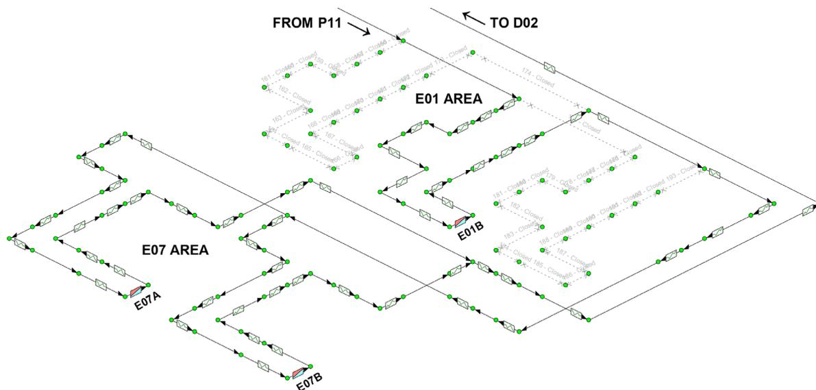
Figure 3: Fragment of the geometry modelled with Pipe Flow Expert, including E01 and E07 heat exchanger zones.
