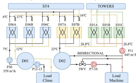
Figure 1: Simplified scheme of the ALBA's thermohydraulic cooling system.
