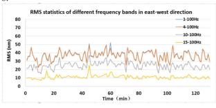
Figure 7: RMS statistics of different frequency bands.
