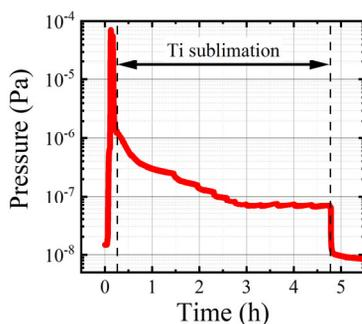
Figure 3: Total pressure curve in the chamber during deposition of the oxygen-free Ti thin film.
