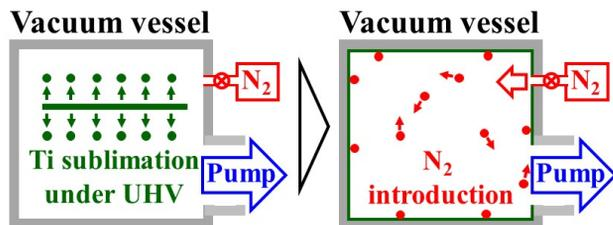
Figure 2: Schematic showing the procedure for deposition of the oxygen-free Ti thin film followed by introduction of high-purity N<sub>2</sub>.
