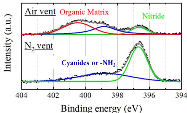
Figure 7: Enlarged SR-XPS spectra in the region of N 1s peaks. Reproduced from Ref. 14, with the permission of Particle Accelerator Society of Japan (PASJ).
