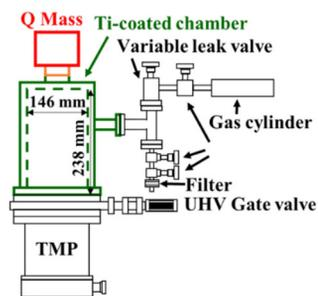
Figure 5: Apparatus for measurements of the total and partial pressures, and mass spectra of residual gases.
