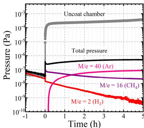
Figure 9: Total and partial pressure curves of the oxygen-free Ti coated vessel for the first cycle of pumping, baking at 185 °C for 6 hours, cooling to RT, and closure of the UHV gate valve. The quadrupole mass spectrometer used was uncalibrated.
