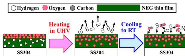
Figure 1: Schematic showing the activation and pumping mechanisms of a NEG thin film deposited on an SS304 stainless-steel substrate.
