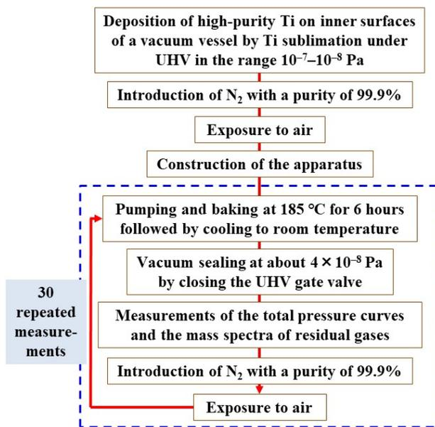
Figure 6: The procedure for 30 repeated measurements of the total pressure curves and the mass spectra of residual gases.
