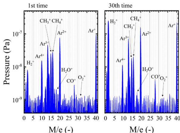
Figure 10: Mass spectra of residual gases after 5 hours of vacuum sealing of the oxygen-free Ti coated vessel for the first and 30th cycles of pumping, baking at 185 °C for 6 hours, cooling to RT, closure of the UHV gate valve, introduction of high-purity N<sub>2</sub>, and exposure to air. The quadrupole mass spectrometer used was uncalibrated.
