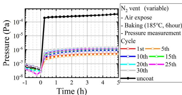
Figure 8: Total pressure curves of the oxygen-free Ti coated vessel as a function of cycles of pumping, baking at 185 °C for 6 hours, cooling to RT, closure of the UHV gate valve, introduction of high-purity N<sub>2</sub>, and exposure to air. Reproduced from Ref. 14, with the permission of PASJ. The quadrupole mass spectrometer used was uncalibrated.
