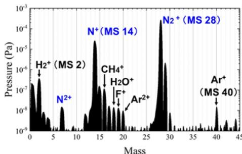
Figure 4: Mass spectrum of introduced high-purity N<sub>2</sub>. The quadrupole mass spectrometer used was uncalibrated.
