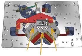
Figure 2: Mirror assembly layout. The yellow circles and arrows show the contact points between mirror and mechanism.
