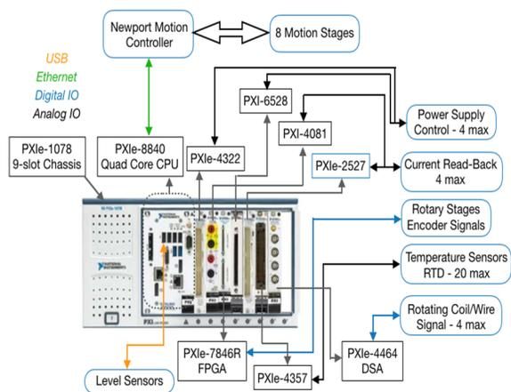
Figure 2: NI DAQ block diagram.
