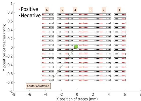
Figure 3: PCB design cross-section showing positive and negative wires of the 6 windings and the rotation center.
