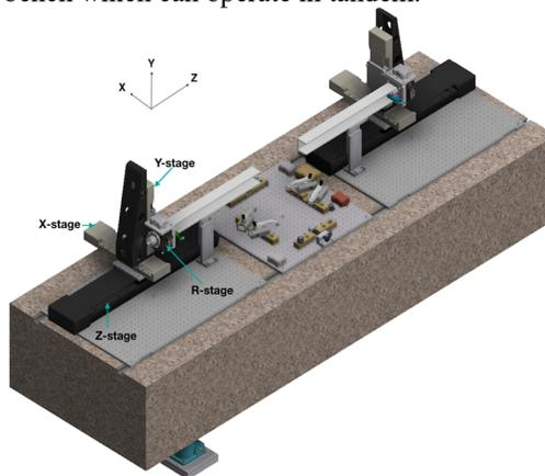
Figure 1: 3D rendering of the NSLS-II magnetic measurement system.
