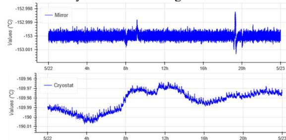
Figure 8: CAT M1 temperature deviation, with maximum values of about 2 mK.
