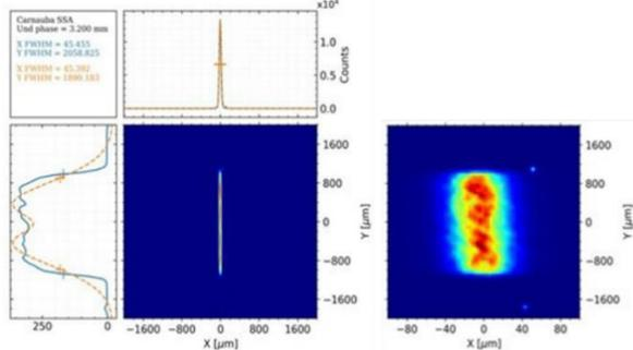
Figure 6: Measurement for the horizontally-focused beam at the CNB beamline, producing a vertical-line beam.
