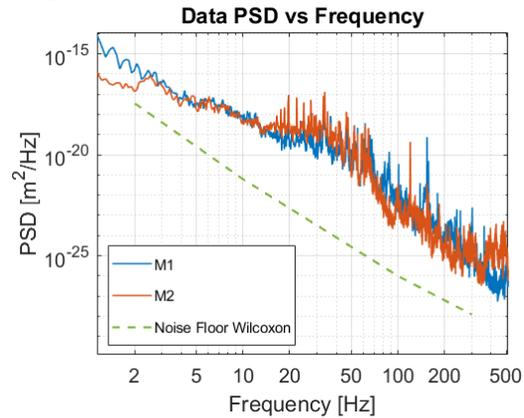
Figure 7: Horizontal displacement Power Spectrum Density measurements for CNB M1 and M2.
