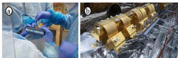
Figure 4: (a) CAT M1 flexible copper braid being fixed to the mirror and (b) the CAR M1 assembly installed inside the UHV chamber.
