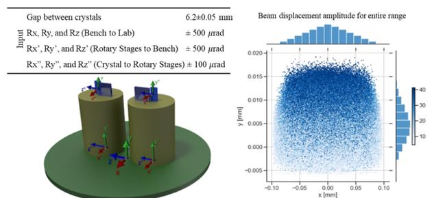
Figure 4: Variations of the virtual source due to random misalignments showed on top-left table.  $1 \times 10^4$  cases were considered inside these ranges. The coordinate systems xyz, x'y'z' and x''y''z'' are fixed to bottom flange, bottom part of goniometers and center of rotation of crystals, respectively.
