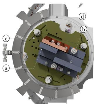
Figure 2: CAD representation of first channel-cut crystal module, containing the first (a) and second (b) diffraction surfaces and the crystal frame (c), which is clamped to the rotary stage (d) at three points 120° spaced.
