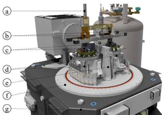
Figure 1: CAD representation of 4CM-CAT. Cryostat (a), copper straps (b), crystals (c), rotary stages (d), linear actuator module (e), vacuum chamber (f), granite bench (g).
