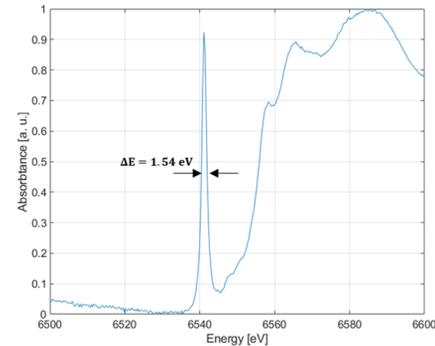
Figure 7: Beamline energy resolution measurement with  $\text{KMnO}_4$  K edge.
