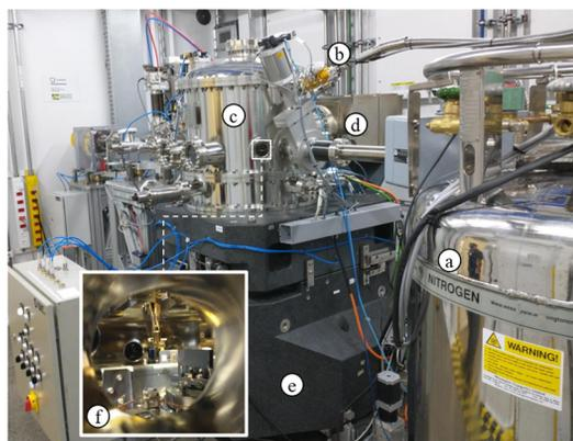
Figure 3: Photography of 4CM-CNB. Liquid nitrogen vessel (a), cryostat (b), vacuum chamber (c), ion pump (d), granite bench (e), and internal view (f).
