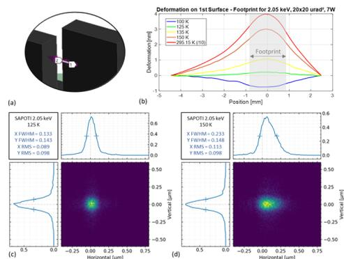
Figure 5: Deformation along the 1st crystal surface of 4CM-CNB (a) due to thermal effects for different bulk temperatures made on Ansys for a  $1.6 \times 2.7 \text{ mm}^2$  7W footprint at 2.05 keV (b). Values for 295.15 K are divided by 10. Raytracing of the diffracted X-Ray beam at experimental station downstream 4CM for crystals at 125 K (c) and 150 K (d) made on Shadow.
