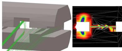
Absorber simulated by using SynRad+. Details of the photon beam trajectory and the footprint of the ID and BM radiation.
