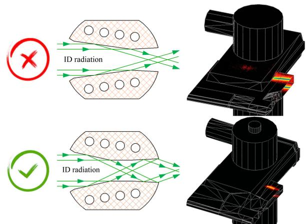
Collision and reflection of the ID radiation vertical mode in a cross section view of the opening. **Upper figure:** The radiation hits the absorber and is reflected directly to the walls of the dipole vacuum chamber. **Lower figure:** After the collision on the absorber the reflected ID radiation hits the internal walls of the Integrated Crotch Absorber.
