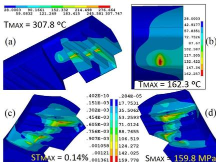
The temperature, stress and strain distribution have been calculated based on linear elastic analysis. The thermal mechanical simulations show good results, the new absorber is in a safe range according to the design criteria. The maximum temperature, stress and strain are 307.8 °C, 159.8 MPa and 0.14%, respectively.
